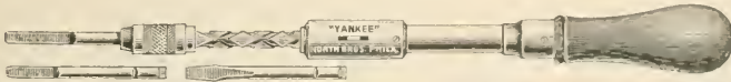
“YANKEE” SPIRAL-RATCHET SCREW DRIVER, No. 30 Drives or takes out screws by pushing on handle, or by ratchet movement. Can be used as rigid screw driver at any part of its length.
