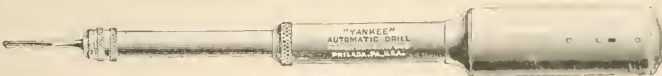
“YANKEE” AUTOMATIC DRILL, No. 40 For boring wood for setting screws, brads, nails, etc; can be used in hard or soft wood without splitting. Pushing on handle revolves drill. Each drill has 3 drill points in magazine inside handle.
